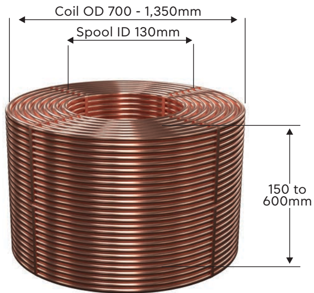
Without carton spool Maximum coil weight: 580kg
